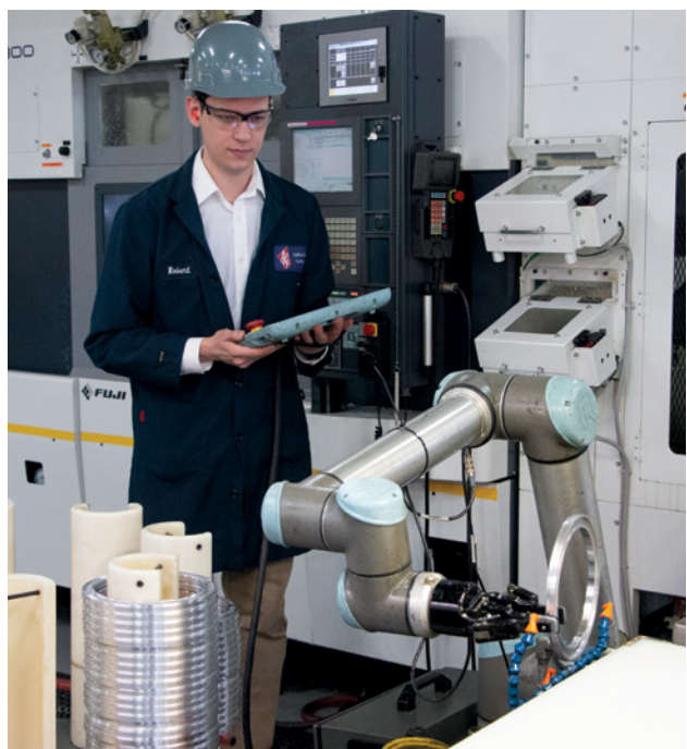
For the machine tending application, RCM Industries typically ran three shifts with three operators running machines on each shift. After implementing cobots, the company was able to reduce that to one person managing all operations in each shift, essentially reducing staffing requirements by six people in that cell.
